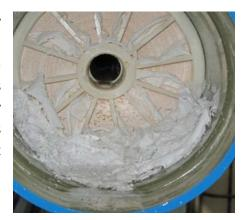
Elements can also be mechanically (compaction, telescoping) or chemically (oxidation, hydrolysis) damaged,
